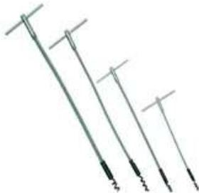
An extraction tool, with long flexible shank to gain access to glands in difficult positions. The corkscrew tips are designed to embed firmly in all types of packing, including badly worn and hardened products.
